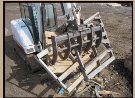
Heavy duty 5 tine rake, with 3/4" thick tines used with excavator thumb to easily rake and pick up debris. 48" Wide, Wt. 350 lb.
