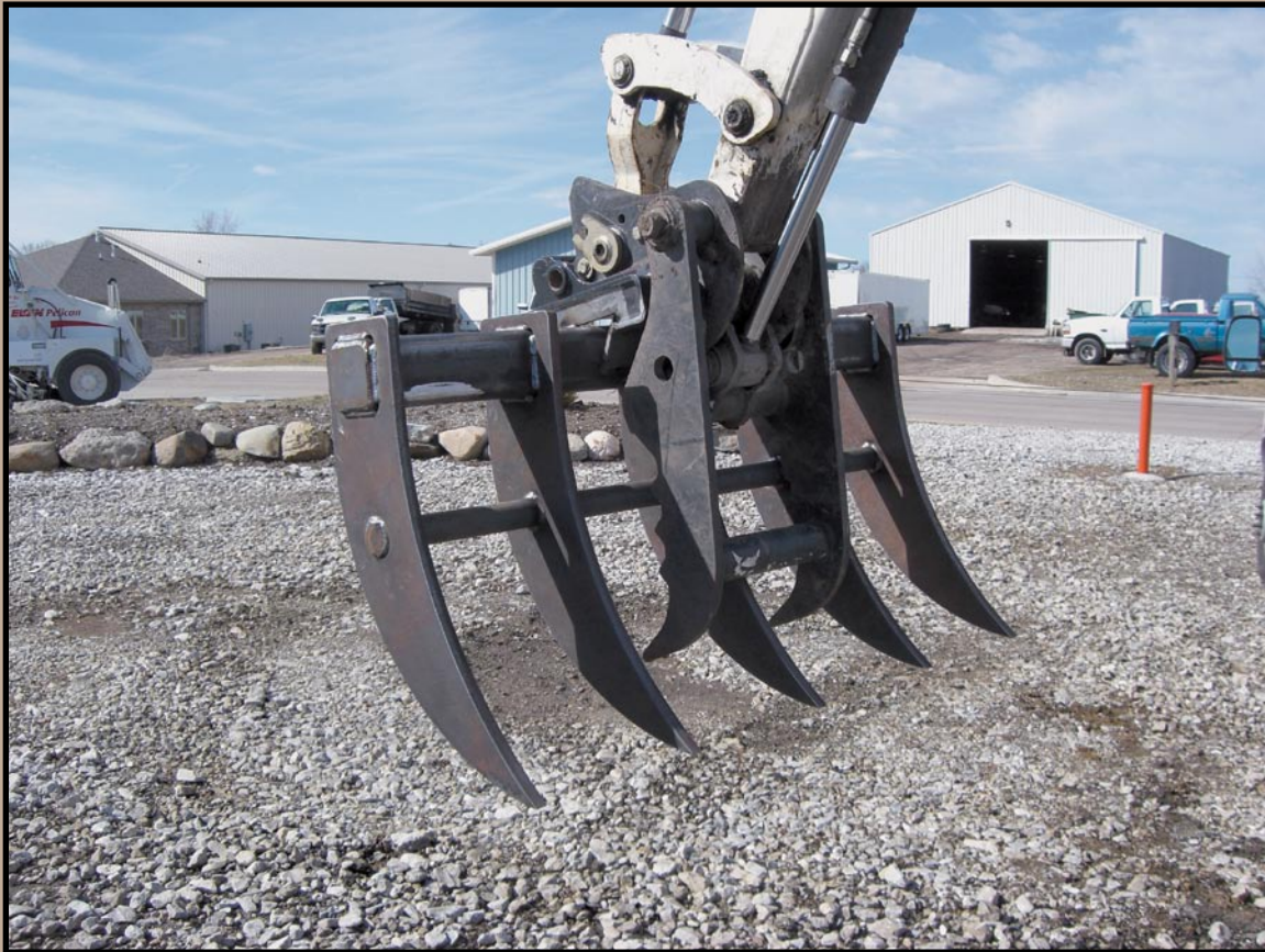
Heavy duty 5 tine rake, with 3/4" thick tines used with excavator thumb to easily rake and pick up debris. 48" Wide, Wt. 350 lb.
